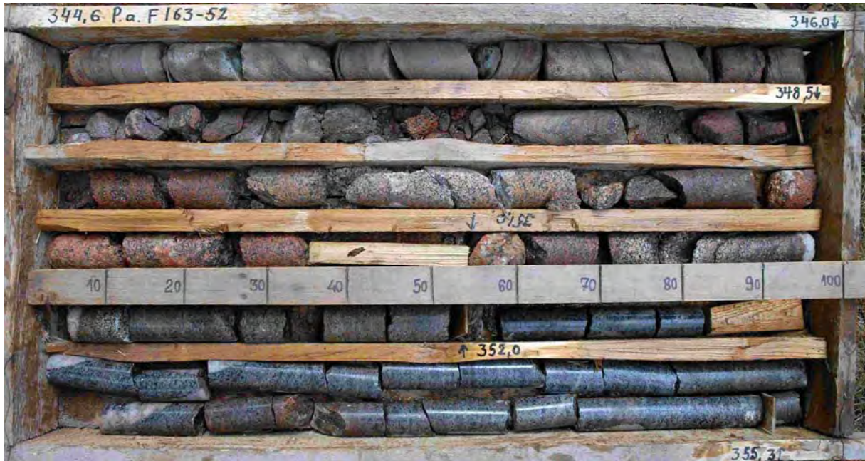
Foto 1.5. Värske (all) ja murenenu (ülal) gneiss puuraugust F163 (Viru-Jaagupi) Photo 1.5. Fresh (below) and weathered (above) gneiss from the well F163 (Viru-Jaagupi)
