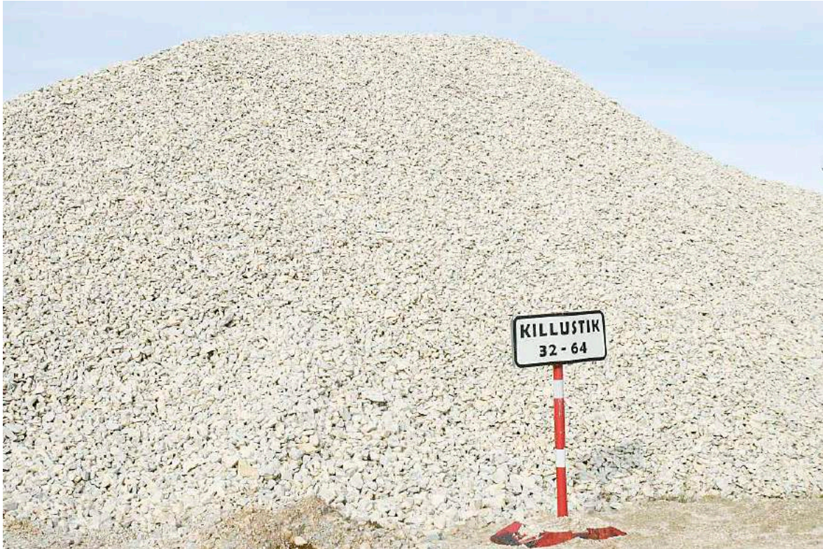
Foto 10. Saunja lubjakivist toodetud killustik Sutlema lubjakivikarjääri. Photo 10. Agregate made from Saunja Limestone in the Sutlema Limestone Quarry.
